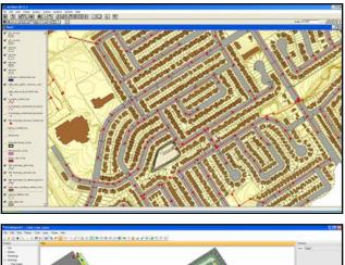
Stormwater management models of the three areas were constructed in **PCSWMM** using existing GIS layers, as-built drawings, and data obtained from field surveys. Precipitation events for a range of return periods from 2 to 100 years were run through the model and flood-prone areas were identified. The simulation results were verified against the City's complaint database from the event as well as through comparison to monitoring data within the study areas.
